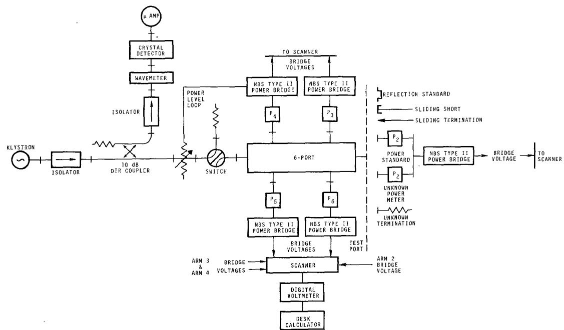
Fig. 2-Block diagram of complete six-port system
