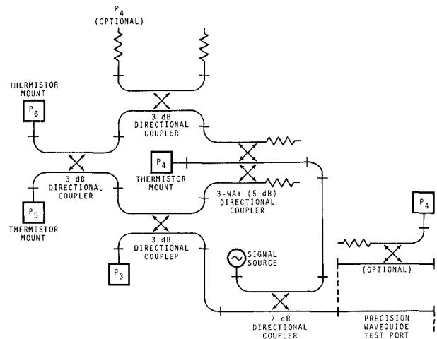
Fig. 1-Six-port waveguide system
